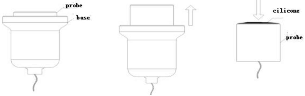
Step2 Apply silicone to the probe
