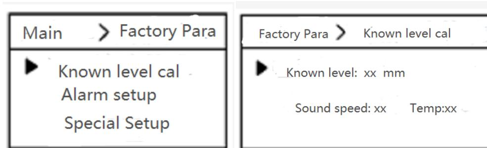
Input the actual measured liquid level as "known level", press "confirm" key.
